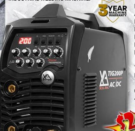
HF ARC START. 2/4T TRIGGER FUNCTION. AC BALANCE AND FREQUENCY CONTROL. PULSE CONTROL FUNCTION. PRE & POST GAS CONTROL. DOWN SLOPE CONTROL. ELECTRODE HOT START & ARC FORCE. DUTY CYCLE @ 40°C 25% @ 200A TIG. 30% @ 160A MMA.
